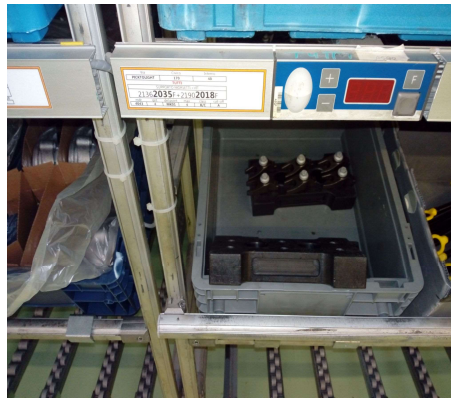
Figure 5-5 – Gravity rack with containers.
