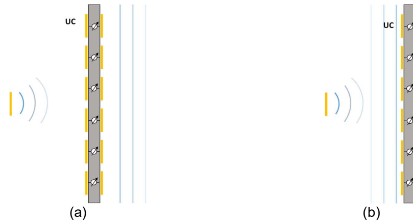
Figure 1.2 – Typical RIS passive architecture: T-RIS/Transmitarray (a), R-RIS/Reflectarray (b)
