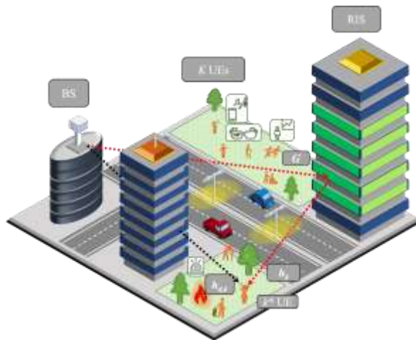
Figure 3-5: Multi-UE RIS-empowered wireless network scenario.
