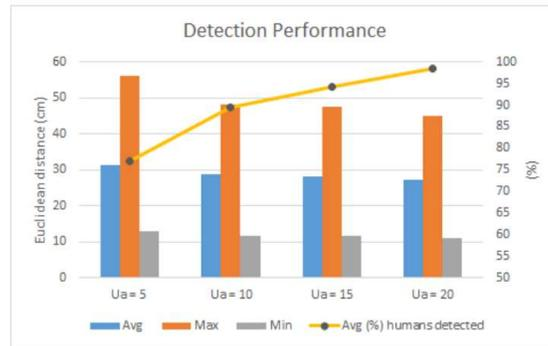
**Figure 6-8: Average human detection percentage (%) and positioning errors (cm) with fixed RIS aperture of  $M = 259 \times 259$ , in a  $\gamma = 0$  dB condition, with  $S = 100$  averaging strategy and  $U_p = 10$  passive users in the scenario for different numbers of active devices  $U_a$ .**
