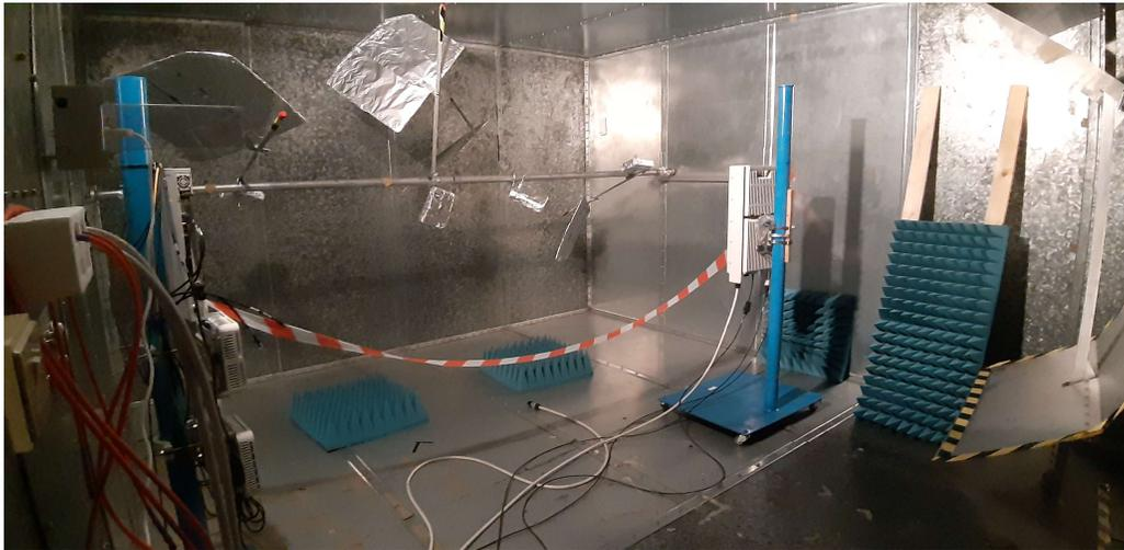
**Figure 2-1. Reverberation chamber used during tests. It is equipped with two stirrers, absorbing materials and, in this case, with the 5G BS module operating at the mm-wave. In addition, on the left side of the chamber there is also the 4G-LTE and 5G (sub-6 GHz) RF modules. Moreover, the user equipment is located within the reverberation chamber and it is connected to a personal computer that collects recorded data.**
