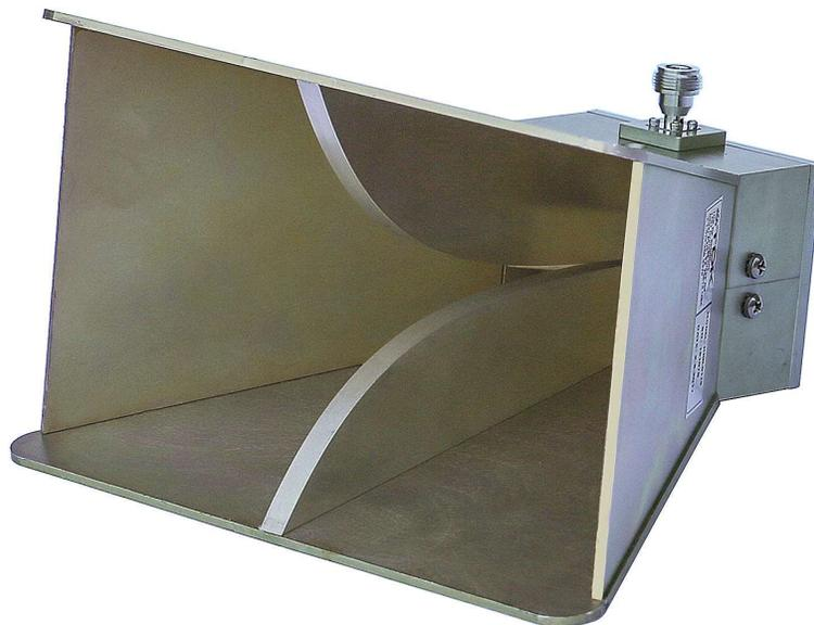
Figure 2-3. Horn antennas
