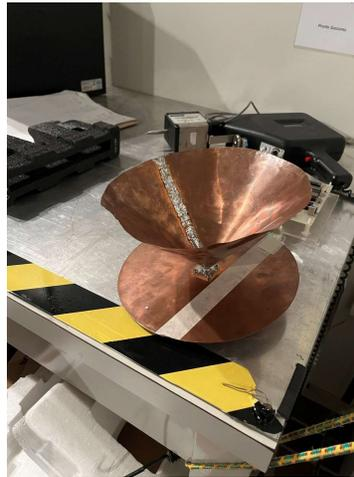
Figure 2-15. Discone antenna RX
