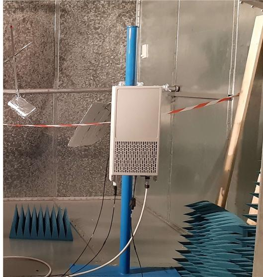
Figure 2-6. mm-waves 5G RF module
