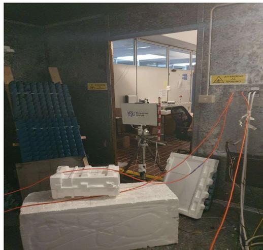
**Figure 2-10. RIS position in the reverberation chamber, in front of the door.**
