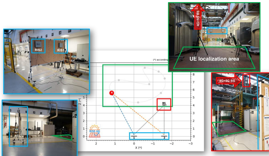
Figure 3-2 The main subareas involved in the trial together with the main elements of the equipment used.
